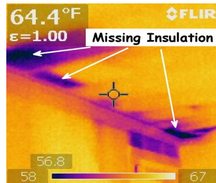
Thermal Imaging Infrared Inspection U.S. IR Inspection Division Contact us for more information
